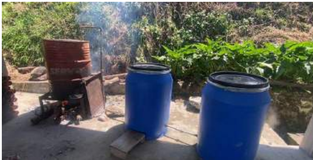
Figure 8: Sterilization drum connected parallel from the steam source
